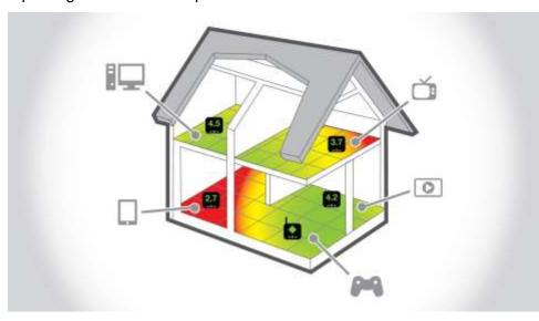
presenting signal levels and channel graphs, the system intelligently selects the best channel, the optimal access point and range extender locations, and provides application level throughput measurements that ensure the Wi-Fi experience meets the needs of the customer. The results are then wrapped up in a birth certificate and uploaded to the cloud for enhanced support services.
